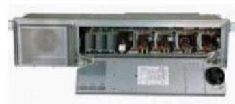
Mitrac<sup>+</sup> TC 1000 Traction Converter for Medium Power Application
